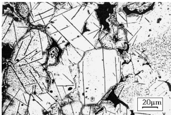
Figure 8 Material B after treatment 1: nitrides of very small dimensions in the interior of the nitrided zone.
